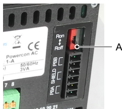
A Switch for terminating resistor
