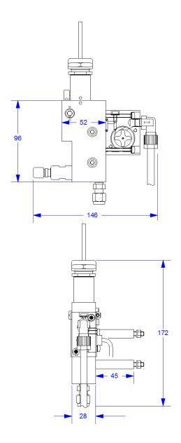
**Delivery:** Flow cell with mounting parts (M5 screws and distance sleeves) for panel mounting.
